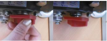
Never activate the red knob when the winch is under load.
