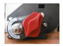
It is essential to remove the winch handle before disengaging the ratchet brake (Red Knob)
