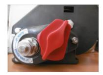
It is essential to remove the winch handle before disengaging the ratchet brake (Red Knob) Never activate the red knob when the winch is under load. Remove the winch handle before activating the red knob. Press in the knob and turn to disengage .
